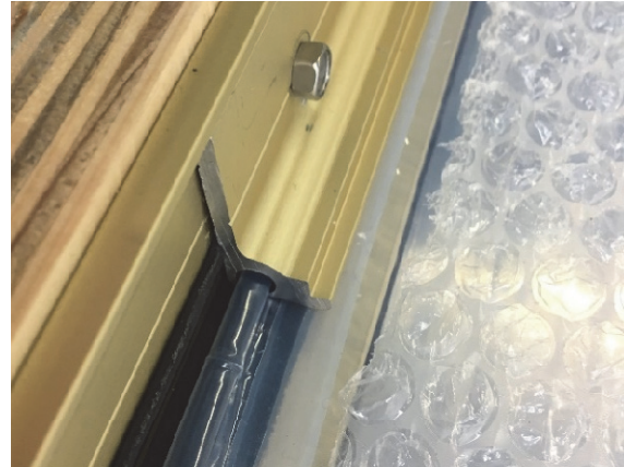
Figure 9: Fixation test of a clamping profile with inserted keder-pocket, ©Taiyo Europe
