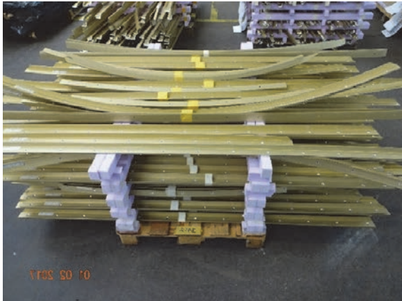
Figure 8: Clamping profiles anodized in a golden tone, straight, pre-bended and pre-twisted, ©Taiyo Europe
