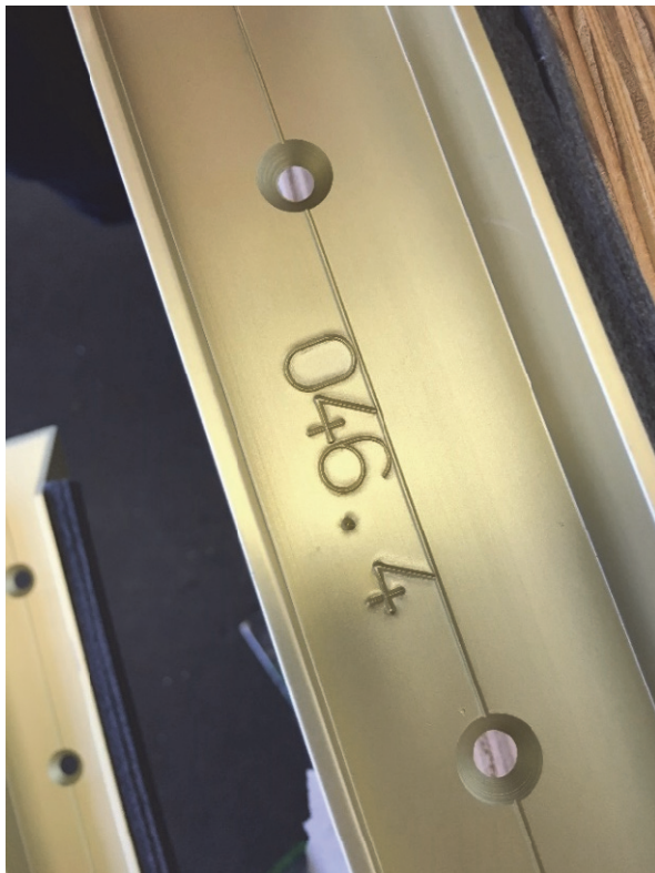
Figure 10: Each profile was given an individual stamped number for correct placement on the component, ©Taiyo Europe
